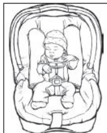
Figure 4. Car safety seat with a small cloth between the crotch strap and infant; chest clip positioned at the center of the chest, even with the infant's armpits; and tightly rolled receiving blankets on both sides of the infant.
